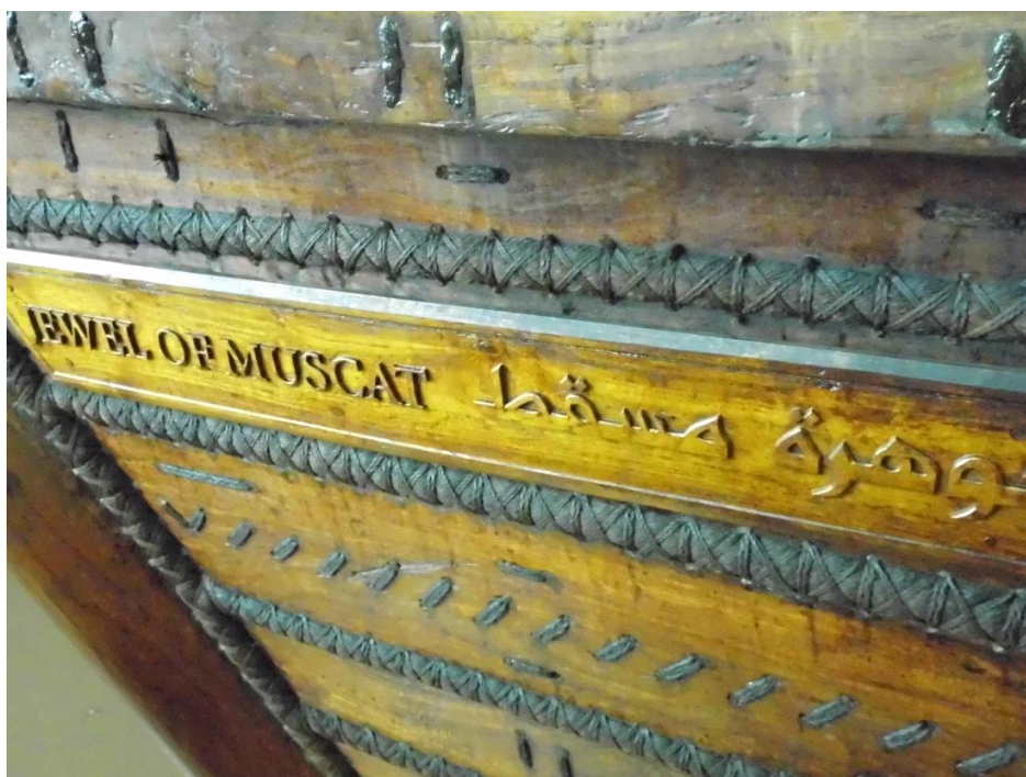
The detailed coir stitching on the Jewel of Muscat on display at the Maritime Experiential Museum in Singapore
